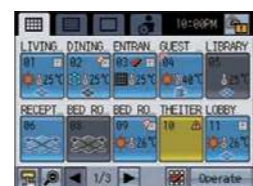
GRID (zoom-in) screen Displays the detailed operation status of each group.
